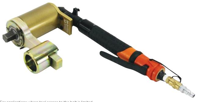
For applications where tool access to the bolt is limited, The RAD SDM Low Profile series multipliers can provide you a solution. Based on RAD's long experience with planetary gear reduction technology, the SDM Low Profile gearbox was designed for confined applications in multiple industries. The RAD SDM Multipliers are to be combined with a nut runner.
